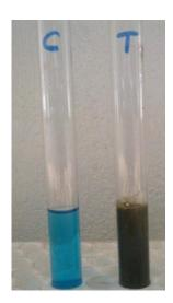
**Figure 2.** Benedicts test – black precipitate obtained.
