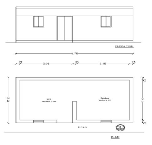
Figure 2. Plan and elevation of low cost house.
