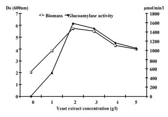
**Figure 5.** Effect of yeast extract concentration on biomass production and glucoamylase activity by *Candida famata*.
