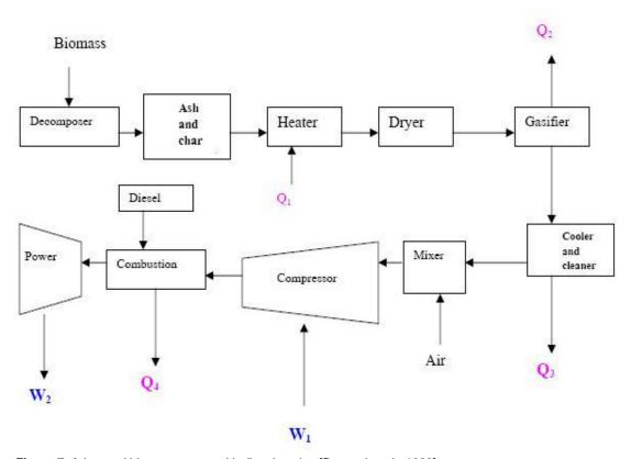
Figure 7. Advanced biomass power with diesel engine [Bacaoui et al., 1998].
