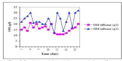
Figure 5. Organic matters before and after treatment in digester [Omer and Yemen, 2003].
