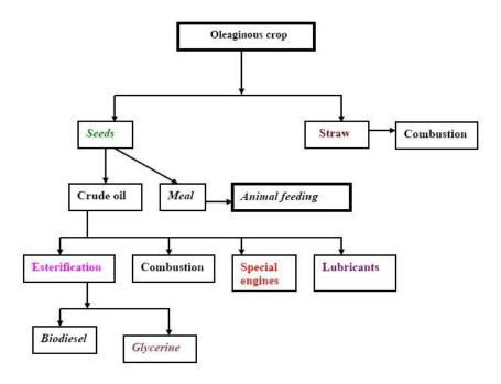
Figure 9. Flow chart of biodiesel production [Hall and Scrase, 1998].
