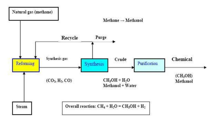
Figure 2. Schematic process flow sheet [Robinson, 2007].
