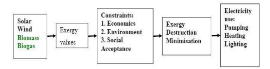
Figure 11. Exergy based optimal energy model [Wu and Boggess, 1999].
