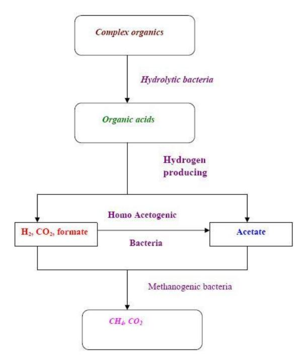
Figure 3. Biogas production processes [Omer and Yemen, 2003].
