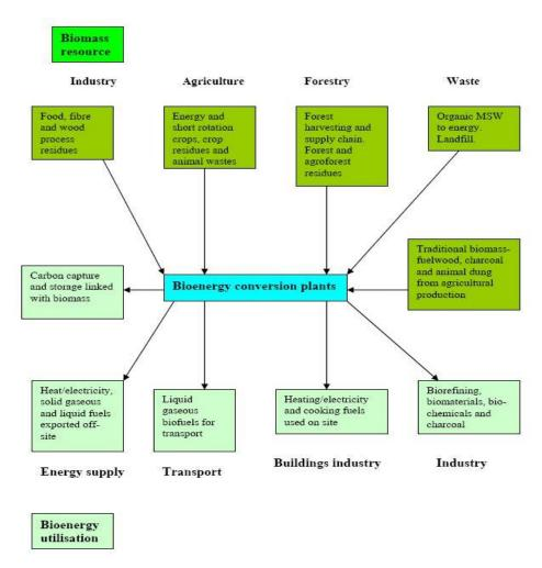
**Figure 4.** Biomass resources from several sources are converted into a range of products for use by transport, industry and building sectors [Omer and Yemen, 2003].
