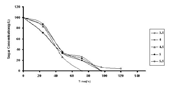
Figure 3. Effect of pH on sugar conversion in fermentation process.
