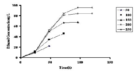
Figure 6. Effect of initial sugar concentration on ethanol production.
