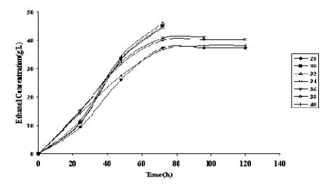
Figure 4. Effect of temperature on ethanol production.
