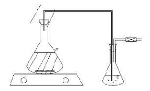
Figure 1. Anaerobic fermentation system for ethanol production.
