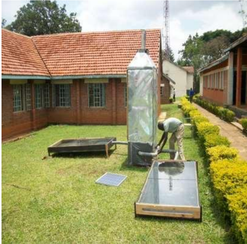
Figure 1. Photographic view of the prototype indirect cabinet solar dryer designed and fabricated at Maseno University, Kenya.
