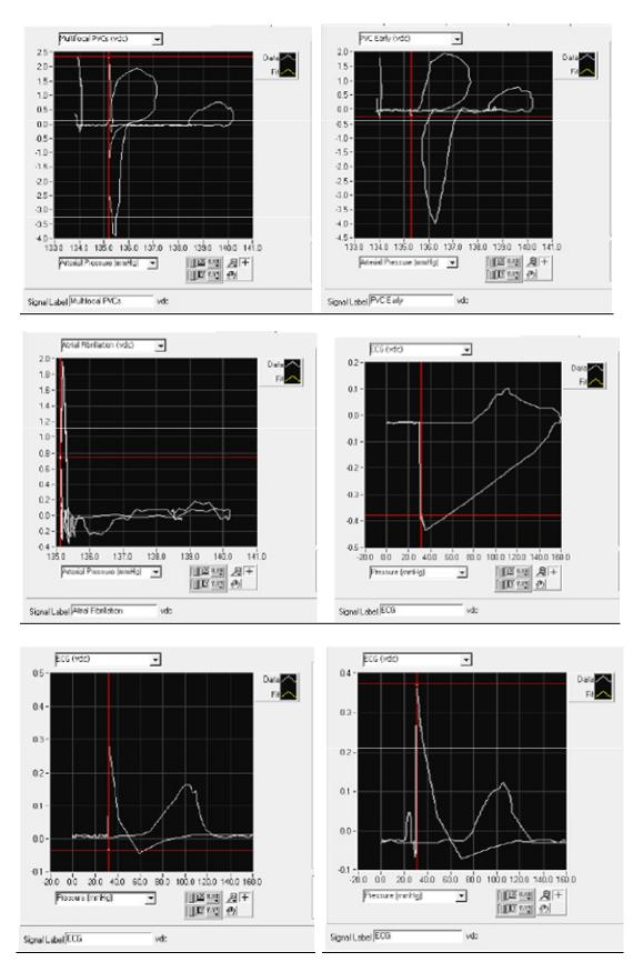
**Figure 12.** VCVGs for cases of a) Multifocal PVC, b) PVC Early, c) Atrial Fibrillation, d) ECG Paced, e) Normal Rhythm (60 bpm), and f) PACs.
