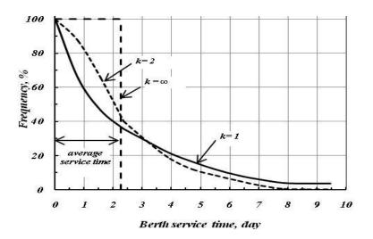
Figure 3. Service time distribution as Erlang Function, hypothetical port.
