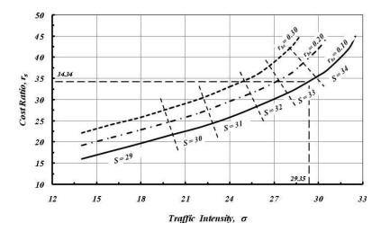
**Figure 8.** Determination of Optimum Number of Berths, due to different cost ratio, rbs, Alexandria Port, Case Study.
