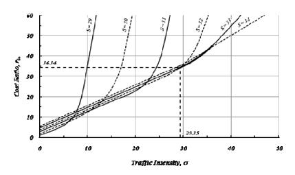
Figure 7. Determination of optimum number of berths, , Alexandria port, case study.
