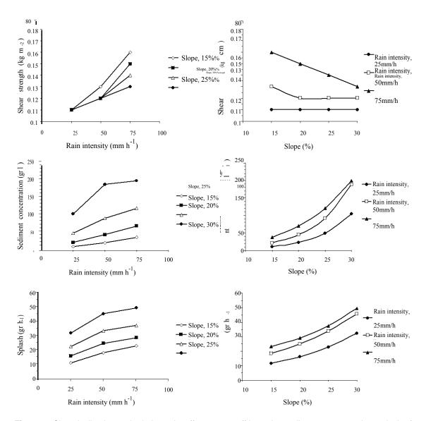
**Figure 3.** Slope inclination and rain intensity effects on runoff intensity, sediment concentration, splash of soil particles in the direction of front section of the flume and shear strength of soil surface in control treatments.
