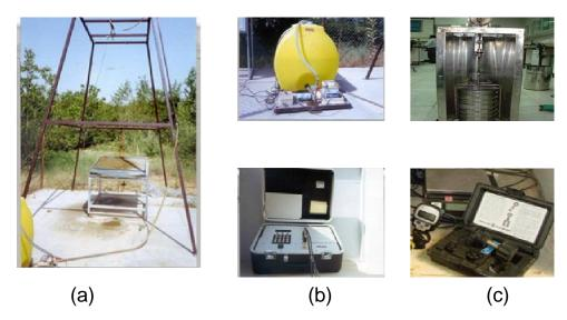
**Figure 2.** The research institute of forests and rangelands of Iran (IRIFR) tilting flume and simulated rainfall facility consisting of: (a) steel frame with oscillating nozzle and tilting flume, (b) water container with water pump (up) and electronic control system (down) and (c) wet sieving apparatus (up) torvane (down).
