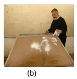
**Figure 1.** (a) five man-maid erosion control materials used in this study and installation of one of them with steel pins and (b) application of PAM and gypsum on the soil surface of the flume.
