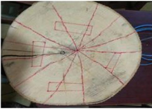
Figure 5. Internal and end checks developed after drying.
