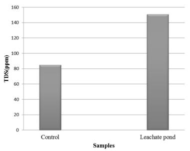
**Fig 4.** Total Dissolved Solids levels of the control water sample and leachate pond watersample in and near Gamodubu landfill.
