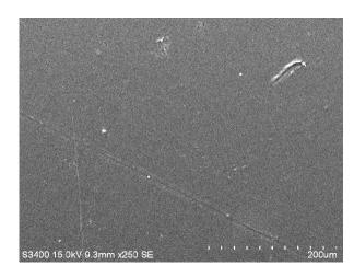
Plate 1. Control untreated LDPE film.
