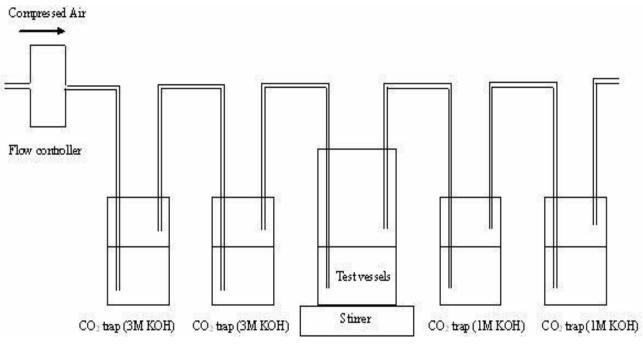
Figure 1. Sturm test.
