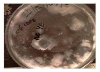
Figure 2. LDPE film showing colonization of hypae.
