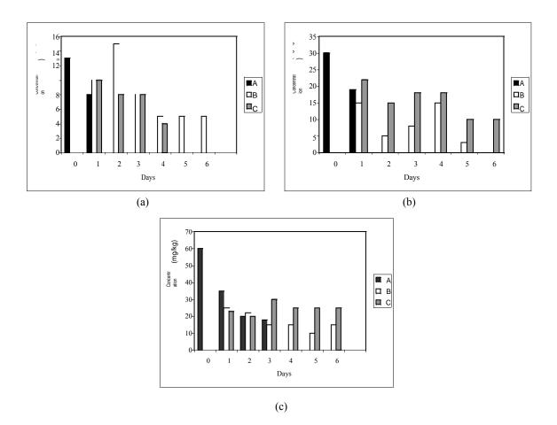
**Figure 2.** Concentration of intermediates found during the bioremediation of chlorpyrifos amended soil (a) 25 mg/l chlorpyrifos amended soil (b) 50 mg/l chlorpyrifos amended soil (c) 100 mg/l chlorpyrifos amended soil where A = Chlorpyrifos, B = Benzyl pyridine and <math>C = TCP.
