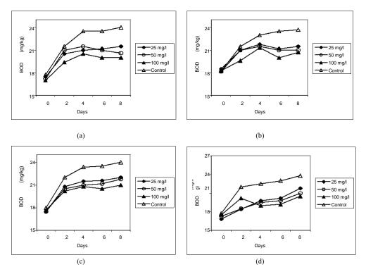
**Figure 7.** Variation in BOD during Bioremediation of pesticide-amended soil in Surface soil treatment unit: (a) Chlorpyrifos amended soil (b) Cypermethrin amended soil (c) Fenvalerate amended soil (d) TBEE amended soil
