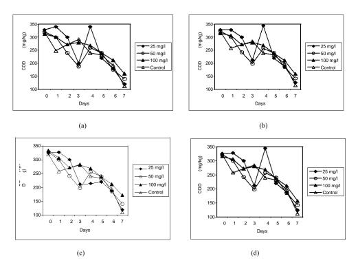
**Figure 6.** Variation in COD during Bioremediation of pesticide-amended soil in Surface soil treatment unit: (a) Chlorpyrifos amended soil (b) Cypermethrin amended soil (c) Fenvalerate amended soil (d) TBEE amended soil
