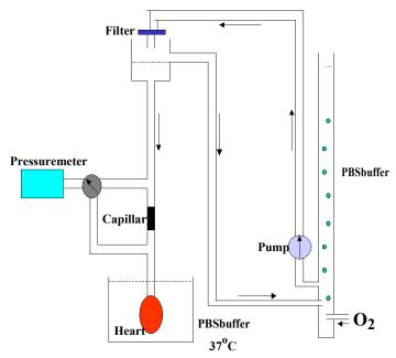
**Figure 1.** Langendorff Heart Preparation Set Up for Coronary Flow Rate Measurement.
