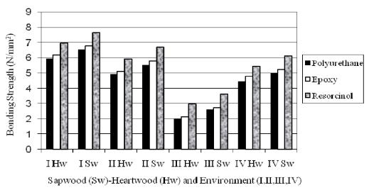
Figures 3. Bonding strength of oak wood according to the environment, sapwood-heartwood, and adhesive type.
