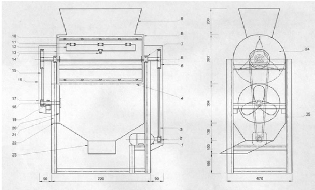
Weight: 90 kg; Overall size = 900 x 470 x 1270 mm; Power Drive: 0.75 hp petrol or diesel engine. Application Potential: For threshing Cowpea and on replacement of beater belts rice, soybeans, sorghum, millet, groundnuts and maize; Advantages: Compact design for easy operation and easy maintenance, highly portable, grain collection feature minimizes spillage, easy collection of biomass and minimum breakage; Status: Research and development stage
