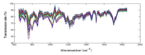
Figure 2. Original transmission spectra of different ibuprofen enantiomers.
