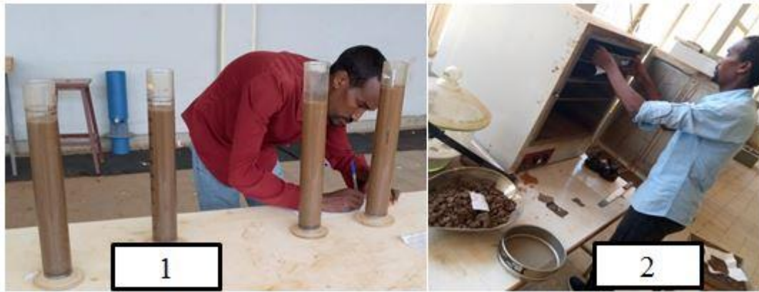
Figure 3. 1 is hydrometer test and 2 is soil oven dry.
