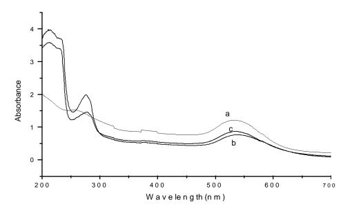
**Figure 3.** UV/Vis spectra of colloidal gold and antibody-gold conjugate. Curve a: colloidal gold solution; curve b: conjugate immediately after addition of antibody to gold solution; curve c: conjugate in buffer after centrifugation and resuspension
