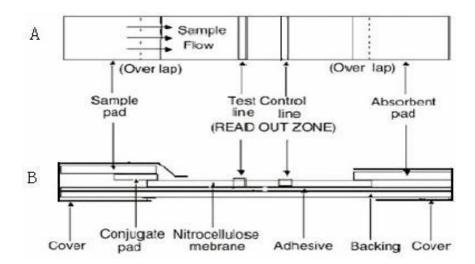
**Figure 1.** Schematic representation of the lateral flow immunochromatographic test strip. (A) Top view; (B) cross-section.
