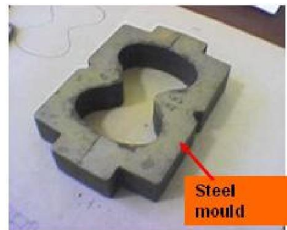
Figure 4. Steel mould used to prepare pull-out sample.
