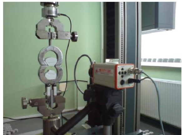
Figure 6. Laboratory pull-out experiment.
