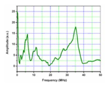
Figure 3. Fourier transformation of the discharge current pulse.
