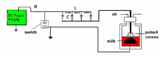
Figure 1. Experimental arrangement and circuit diagram of the hybrid gas-liquid electrical discharge system.
