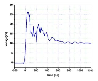
Figure 2. Typical discharge current and the voltage waveforms.
