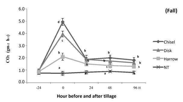
Figure 2. Soil  $CO_2$  flux associated with fall tillage treatments (for the same hour, treatments with the same letter are not significantely differents, (LSD test, p<0.05).
