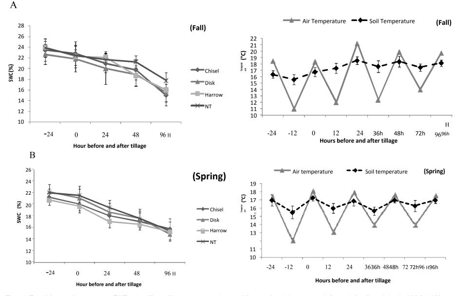
Figure 4. Topsoil (0 to 5 cm) water content (SWC) under different tillage treatments and mean soil (0 to 5 cm) and air temperature before and after tillage during the (a) fall and (b) spring. (\*) means the presence of significant differences between treatments.
