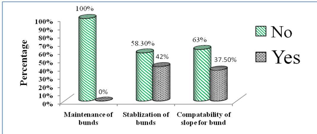
Figure 2. Evaluation result of soil bunds interms of maintenance, stability and compatibility.
