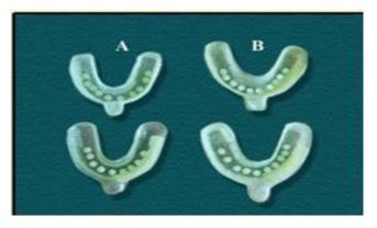
**Figure 7.** (A) Composite and (B) Compomer pellets subjected to bleaching treatment before microhardness evaluation.
