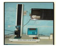
Figure 10. Universal testing machine.
