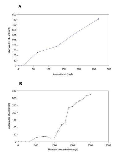
**Figure 2**. Effect of ammonium-N (A) and nitrate-N (B) on phenol biodegradation by Ca-alginate immobilized cells of *Acinetobacter* sp. strain W-17 in simulated wastewater medium (SW).
