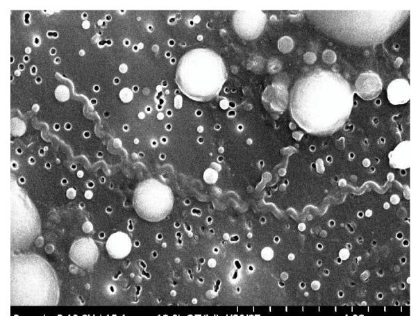
**Figure 4.** Leptospira spirochetes on the surface of a 0.22- m pore diameter filter (Durapore Polyvinylidene fluoride membrane). Surface of filter indicate overlapping pores that could be large enough to allow passage of leptospires under vacuum (Bar, 4.0 m).
