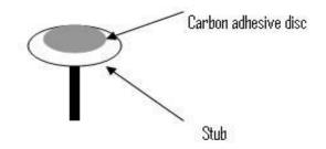
Figure 2. Environmental scanning electron microscope stub.
