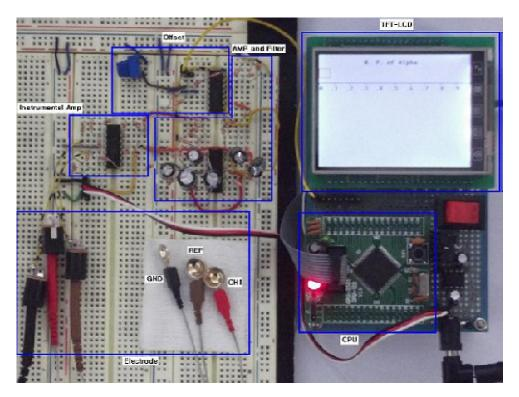
**Figure 5.** Real-time 1-channel embedded EEG measurement system for the finally designed emotion recognition.
