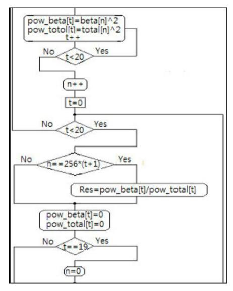
Figure 4. State diagram that monitors the relative power for 20 s.
