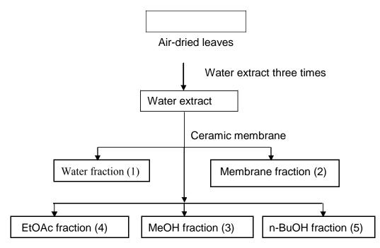
Figure 1. The chart of extraction process.
