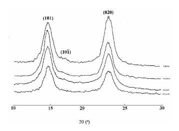
**Figure 5.** X-ray diffraction pattern of the BCs from top to bottom, Glucose, fructose, inositol and glycerol.
