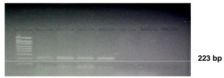
**Figure 13.** PCR amplification of *Brucella* species DNA from aborted bovine fetus samples using (B4, B5) primer set. Lane 1: 100 bp marker; lane 3 to 5: Positive field samples; lane 6 to 7: Negative field samples; lane 2: positive control and lane 8: Negative control.
