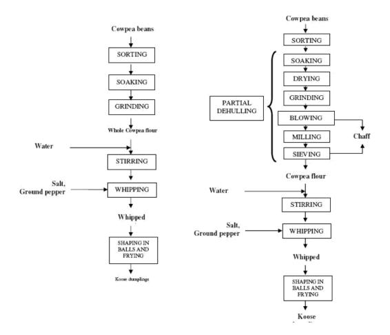
Figure 4. Flow diagrams for koose processing.
