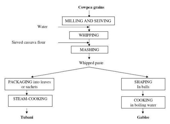
Figure 3. Flow diagrams for tubani and gablee processing.
