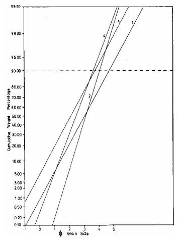
Figure 7. Probability plot based on results of sieve analysis of samples. Note position of d<sub>10</sub> of samples.
