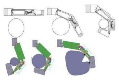
$\label{eq:Figure 2.} \textbf{Figure 2.} \ \ \text{Grasp simulation of underactuated robot finger with the mechanism in Figure 1a.}$
