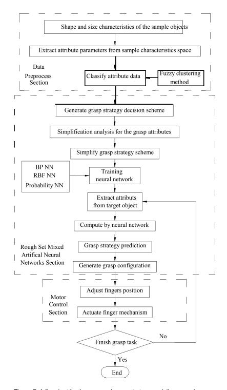
**Figure 7.** A flowchart for the proposed grasp strategy modeling procedure.
