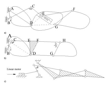
Figure 1. Three kinds of finger mechanisms for underactuated robot hand.
