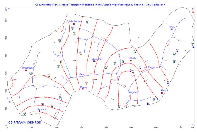
Figure 9. Computed groundwater level contours in m (amsl) and velocity vectors in the 2<sup>nd</sup> layer – February 2008
