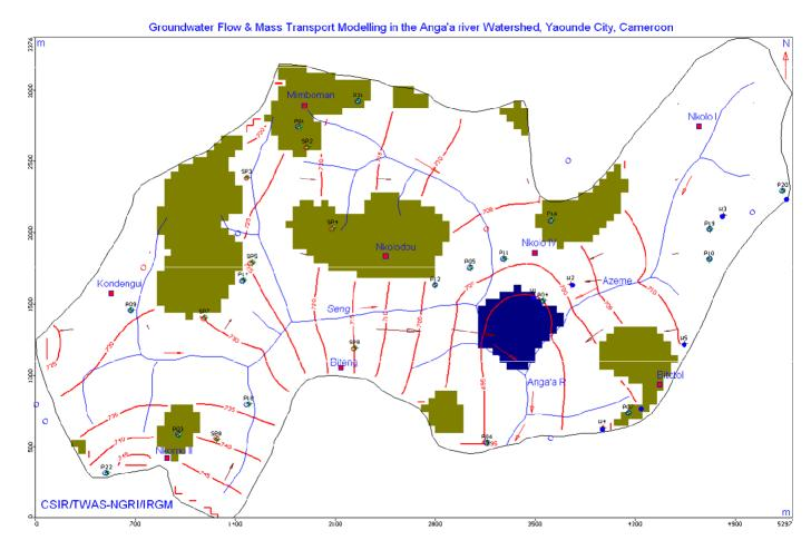
Figure 8. Computed groundwater level contours in m (amsl) and dry cells in the 1<sup>st</sup> layer – February 2008.
