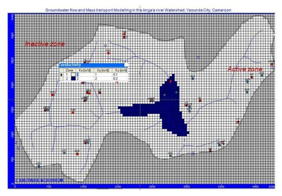
**Figure 4.** Discretization of the simulated Model domain, Active and Inactive Flow Zones and Simulated Hydraulic Conductivity distribution (in m/day) in Groundwater Flow Model.
