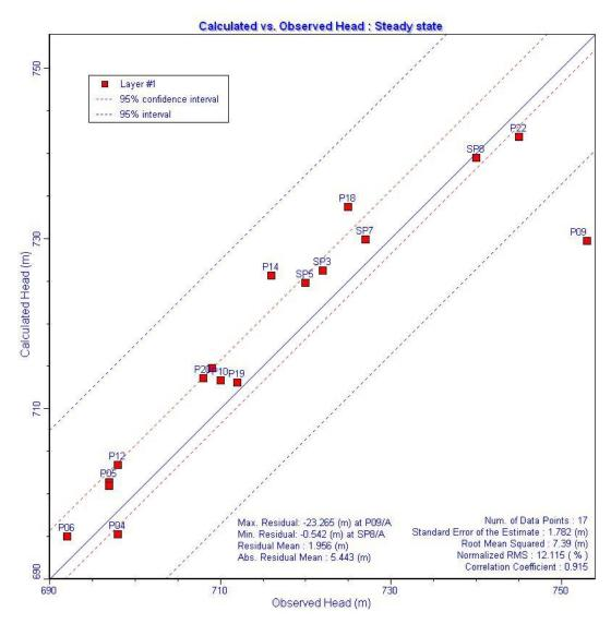
**Figure 7.** Comparison of computed vs. observed groundwater levels in the Anga'a river watershed (February 2008).
