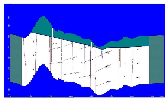
Figure 10. Computed groundwater table cross section and velocity vectors along Row 35.
