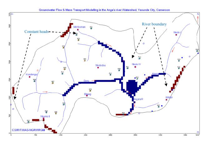
Figure 5. Constant head and river boundary conditions in the flow model.
