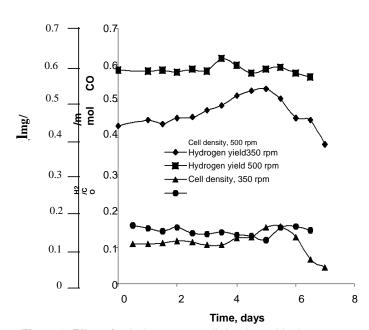
**Figure 3.** Effect of agitation rate on cell density and hydrogen production in continuous fermentation
