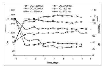
**Figure 6.** Effect of light intensity on H<sub>2</sub> production and CO reduction with continuous culture.
