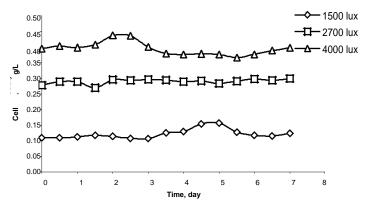
**Figure 5.** Effect of light intensity on cell density in continous fermentation
