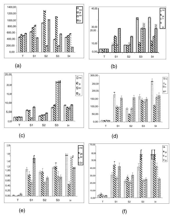
**Figure 2.** Available concentrations (mg/kg) of Fe (a). Cu (b). Ni (c). Zn (d). Cd (e). Pb (f) in cultivated soils (no = november; ja = january; av = april; ju = july; T = Control; S1 = Camp Prison; S2 = Norvegien; S3 = Douze Poteaux; S4 = Sabongari Gare)
