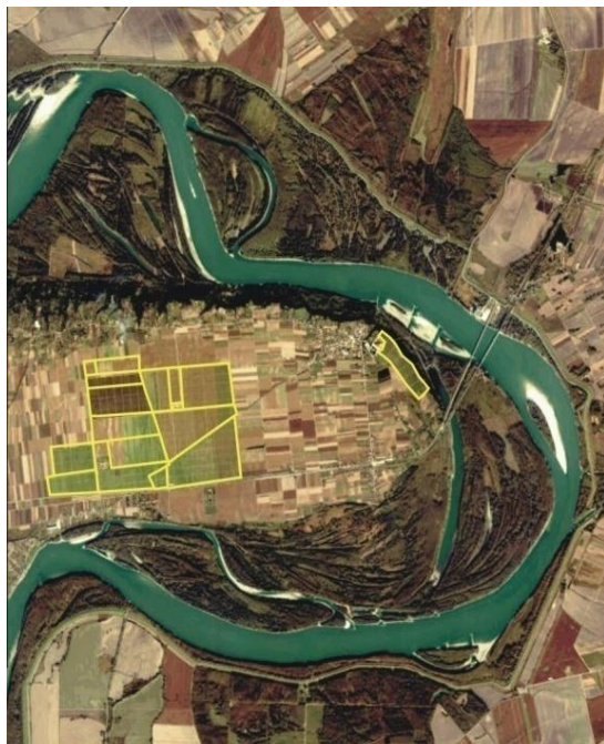
Figure 5. An example of Ikonos image, 1 m resolution, which can be used to make fast inventory of vineyards (Erdut vineyards outlined in yellow).
