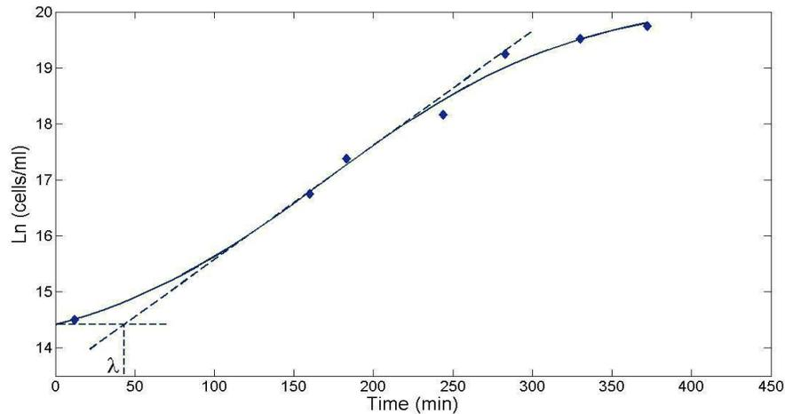
**Figure 2.** Cell concentration (experiment C), measured with the flow cytometer using an internal calibrator. A sigmoid curve has been fitted ( $r^2 = 0.993$ ). The lag phase calculated by means of the geometrical definition is  $\lambda = 43\text{min}$ .
