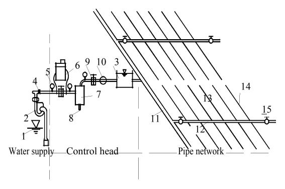
**Figure 1.** Micro-pressure drip system components. 1 = pump; 2 = water supply; 3 = pressure regulator; 4 = back-flow prevention valve; 5 = pressure valve; 6 = fertilizer injecting device; 7 = filter; 8 = waste-drain valve; 9 = valve; 10 = flow meter; 11 = mainlines; 12 = manifolds; 13 = laterals; 14 = emitters; 15 = flush-out valve.
