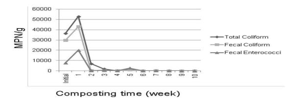
Figure 4. Indicator microorganisms count during composting time.
