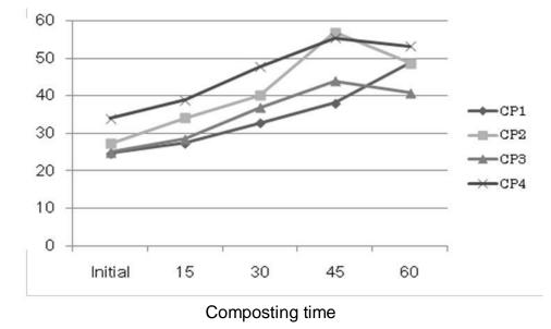
Figure 2. Temperature profile during composting time.
