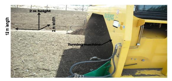
Figure 1. Pictorial view of windrow composting cattle manure piles during turning.
