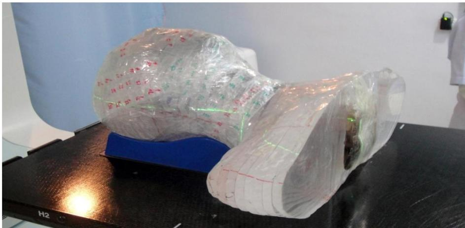
**Figure 2.** Anthropomorphic Perspex head and neck phantom after loading with TLDs.
