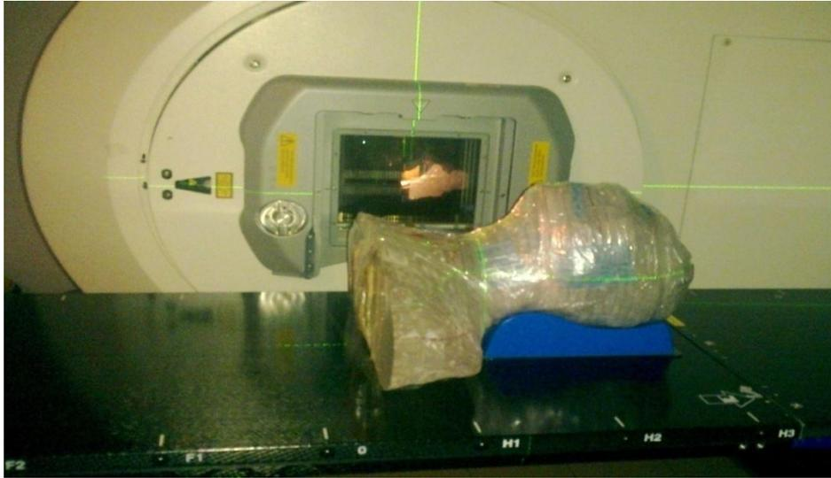
**Figure 4.** Anthropomorphic Perspex head and neck phantom during IMRT treatment.
