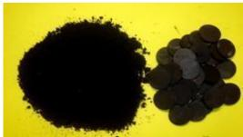
Density =  $0.95 - 1.30 \text{ g/cm}^3$ Porosity surface area (S<sub>BET</sub>) =  $680 - 1123 \text{ m}^2/\text{g}$ Micropore surface area (S<sub>MICRO</sub>) =  $360 - 1016 \text{ m}^2/\text{g}$
