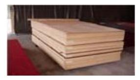
Plate 3. Plywood from oil palm trunk.
