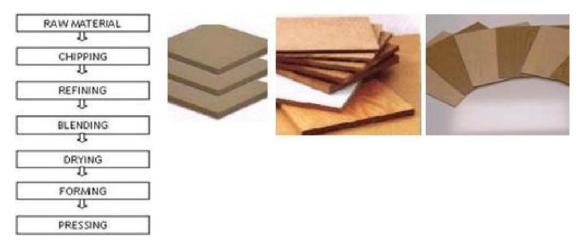
Figure 1. Flow chart of the MDF manufacturing and samples of MDF.
