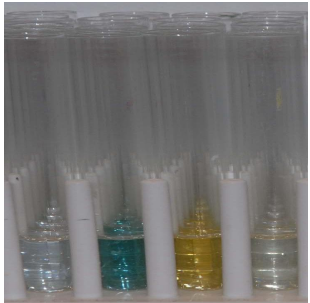
Figure 3d. Fractions collected after gel filtration chromatography of "green fractions" (pool 56-60), the blue fractions are pure laccase.
