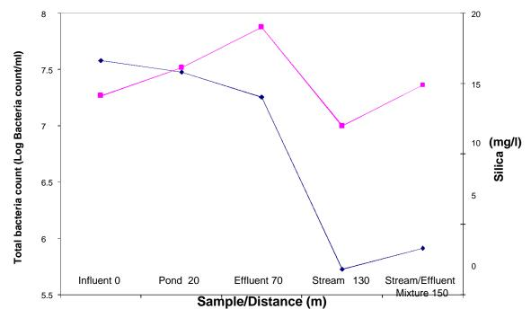
**Figure 7.** Relationship between total bacteria count and silica content in a sewage oxidation pond. Each sample point is the mean of 4 replicate analysis.
