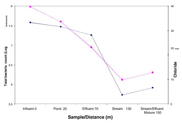
**Figure 6.** Relationship between total bacteria count and chloride content in a sewage oxidation pond. Each sample point is the mean of 4 replicate analysis.
