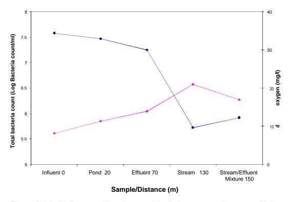
**Figure 3.** Relationship between total bacteria count and dissolved oxygen content in a sewage oxidation pond. Each sample point is the mean of 4 replicate analysis.
