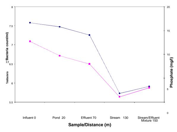
**Figure 5.** Relationship between total bacteria count and phosphate content in a sewage oxidation pond. Each sample point is the mean of 4 replicate analysis.
