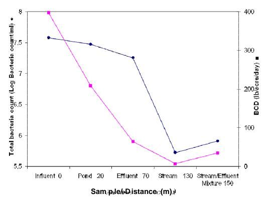
**Figure 2.** Relationship between total bacteria count and biochemical oxygen demand (BOD) in a sewage oxidation pond. Each sample point is the mean of 4 replicate analysis.
