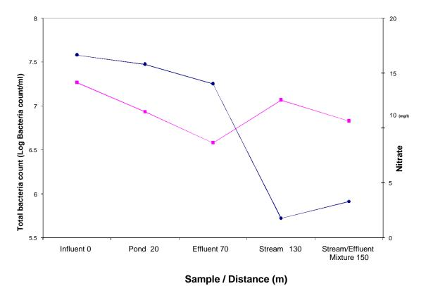
**Figure 4.** Relationship between total bacteria count and nitrate content in a sewage oxidation pond. Each sample point is the mean of 4 replicate analysis.
