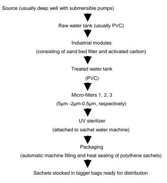
Figure 3. Typical water treatment process in sachet water factories.
