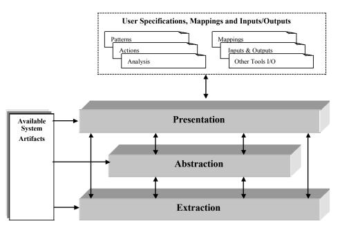
Figure 7. High-level reverse engineering process.
