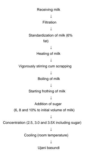
Figure 1. Flow diagram of product manufacture.
