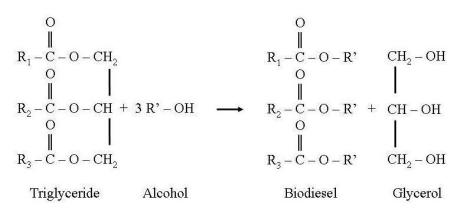
Figure 3. Schematic representation of the transesterification reaction.
