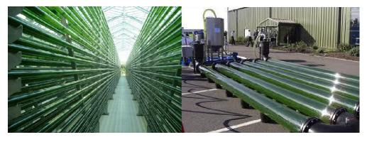
**Figure 5.** Technology for production of microalgae in tubular photobioreactors. Source: Calpoly (2011).
