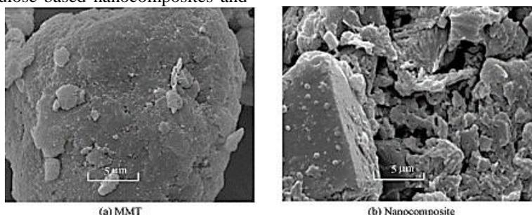
**Figure 6.** SEM image of Montmorillonite (MMT) and nanocomposites.
